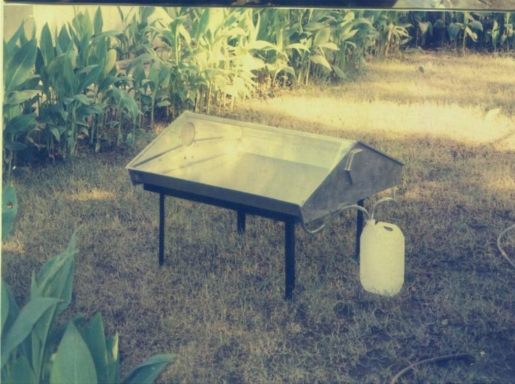
Utilizing solar energy, vaporizing tables or pools, and distillation piping/collection, families and small communities can do a LOT on their own to produce distilled/clean water. Solar energy does not imply “high tech” - ancient people used passive-solar or design-solar (how they build and arranged their living spaces) to take advantage of the sun in heating and to avoid its impacts in the summer.
